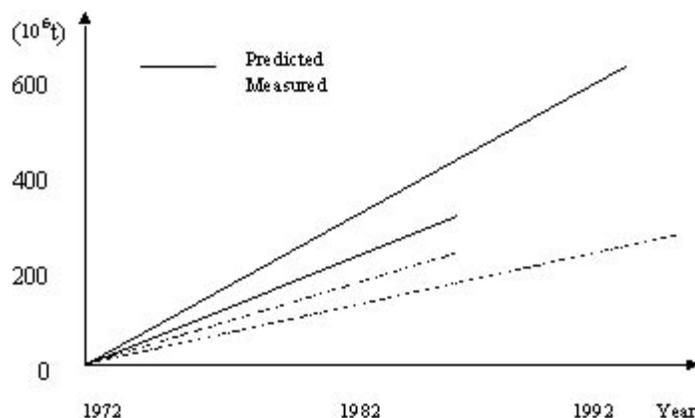
**Figure 2.** Predicted and measured depositional effects in the Iron Gate I HPP reservoir
